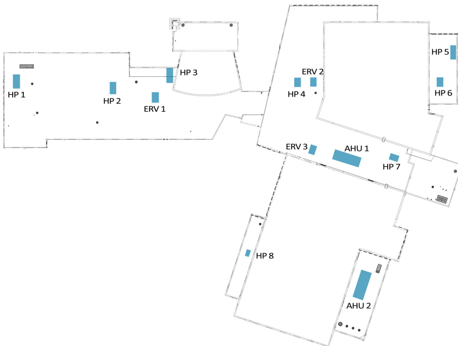
Figure 12 – New Roof Layout
